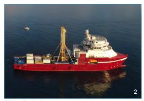
Dina Polaris Arranged for X377, 2022 MSPs capable of deploying up to 3000 m of drill pipe
