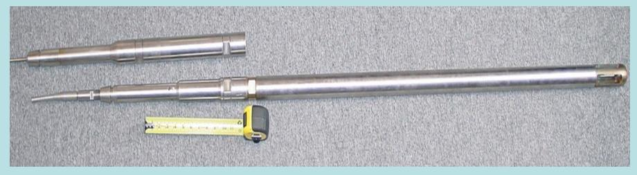
Perma Works is currently offering a 300C analog tool for monitoring pressure, temperature and flow inside geothermal wells.
