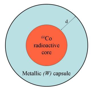
The outer sphere, or capsule, needs to be made of mechanically strong, dense, refractory material. Its main functions are to protect the inner sphere (the heat source), conduct the heat efficiently to the outer surface of the probe and provide weight.
