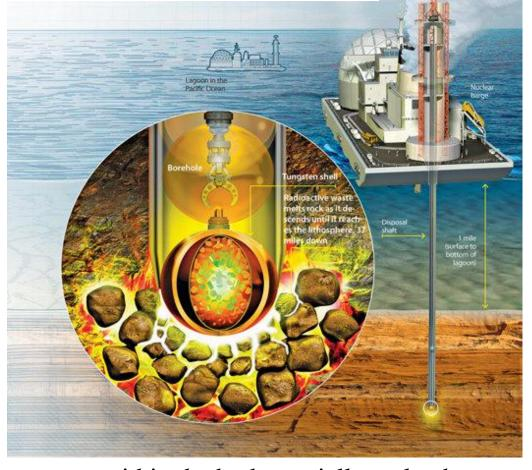
The mechanism is simple. Heat from a source within the body partially melts the enclosing rock and the relatively low viscosity and density of the silicate melt allow it to be displaced upwards past the heavier body as it sinks (Emerman and Turcotte 1983). Eventually the melt cools and vitrifies or recrystallizes, sealing the route along which the body passed.
