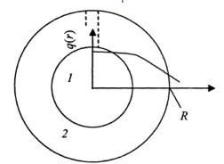
Fig. 1. Form of a self-sinking capsule: I) active material; 2) capsule; q(r) – distribution of heat sources in the capsule.
