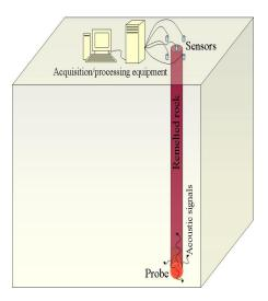
The acoustic signals generated during the melting and subsequent recrystallisation of the rocks through which the probe descends could be detected at the Earth's surface. These signals could provide valuable information about the physical properties of the rocks and uniquely define the mineralogical and chemical compositions and other properties of the rocks.
