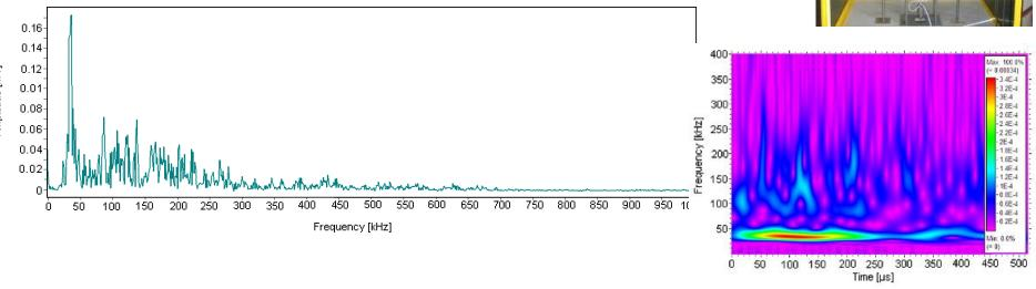
The signals associated with the granite melting-crystallization were distinguished from the equipment noise on the basis of their primary frequencies of **39 kHz** and in the range between 101 and 300 kHz, particularly at 249, 244, 283, 205 and 112 kHz.
