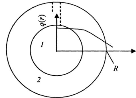
Fig. 1. Form of a self-sinking capsule: 1) active material; 2) capsule;  $q(r)$  – distribution of heat sources in the capsule.
