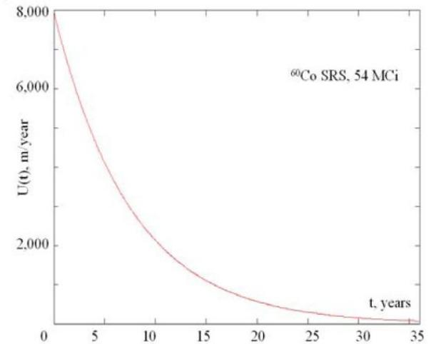
**Fig. 3. Penetration depth (km) of a self-descending 50-cm radius tungsten capsule heated by <sup>60</sup>Co SRS (a) and the rate of self-burial (b).**
