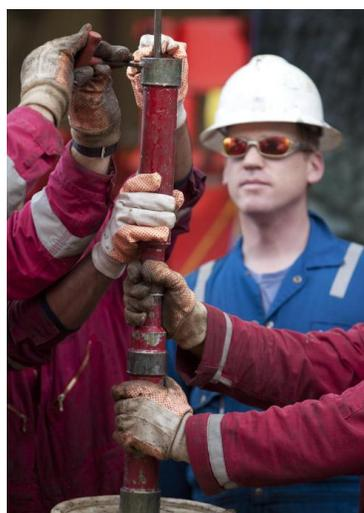
From back to front, Bong Gobalane (Floorman, Siem Offshore), Brad Weymer (Curatorial Specialist, IODP-USIO/TAMU) and Erik Moortgat (Chemistry Laboratory Technician, IODP-USIO/TAMU) patiently wait for core to be pumped out of a stuck liner.
