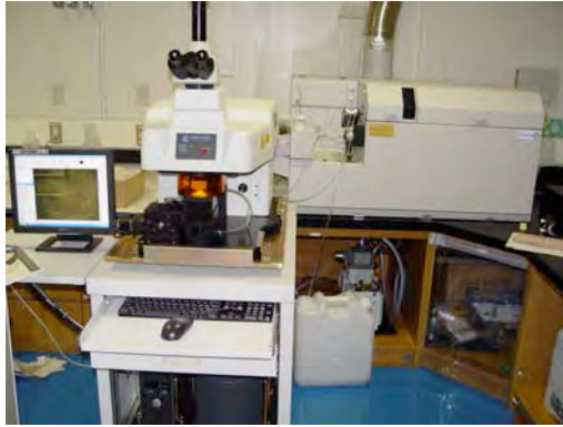
NEW WAVE RESEARCH UP213 system Nd-YAG Laser with 213nm wavelength
